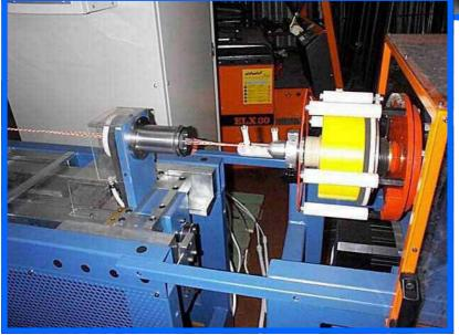
The concentric bending head must be located near the SZ head to stop the lay lenght
